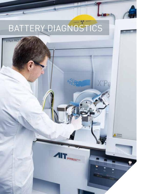
Battery diagnostics include electrical testing of cells under normal and abuse conditions, measuring of structural changes in electrode materials, in operando gas analysis of electrolytes, and contactless expansion measurement of cells. The combination of electrochemical and morphological characterisation results in a comprehensive diagnostics portfolio.
