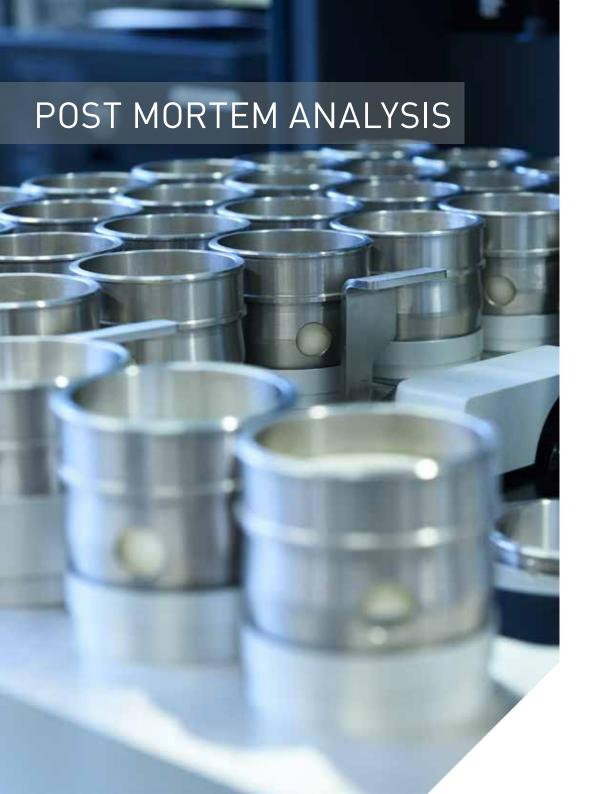
For investigating and understanding electrode degradation, commercial or self-produced cells are opened and disassembled in a glove box under inert gas conditions (Argon). In-house analytics enable elemental and structural analyses and investigation of the morphology of cell components and the condition of components (electrodes and separator) can be evaluated. The results flow directly into ageing simulations.
