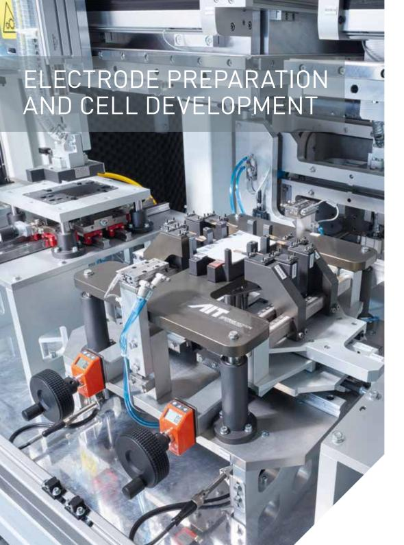
Our Dry Room, together with a modern research pilot line for the production of stacked pouch cells, enables us to perform industrially relevant protoyping. Special attention is paid to the optimisation of each individual production step.
