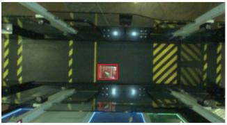
Figure: Visualization of a detected left object (magazine) indicated by a red bounding box
